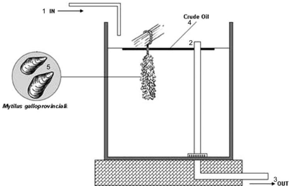
Figure 1. Schematic representation of the microcosm systems used in this study. (1) Tube for water filling, (2) overflow system for discharge of excess seawater, (3) system for seawater outflow, (4) crude oil, (5) *Mytilus galloprovincialis*.
